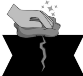
Gambar 8. Excess Penetrant Removal [7]
