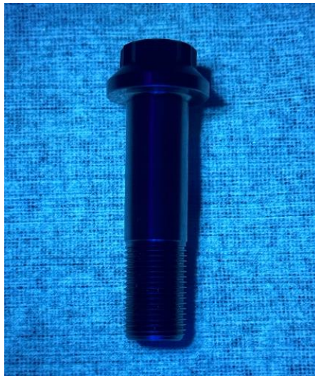
Gambar 15. Post-inspection engine mount bolt
