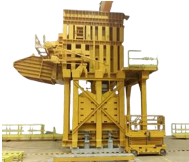
Gambar 2: Trial Fit Structure Chute Gallery, GBC Chute
