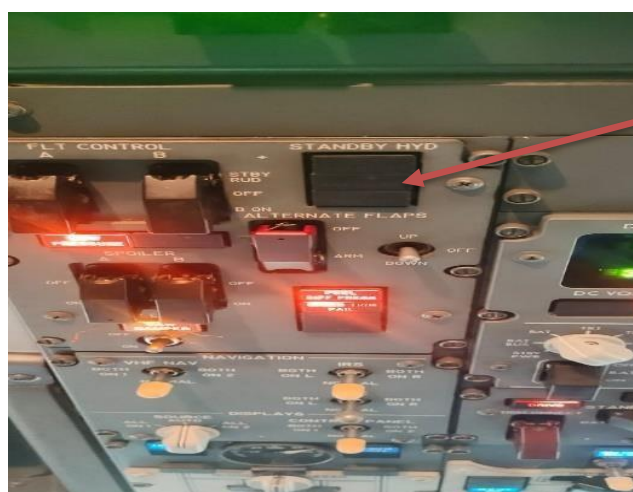
Gambar 9. Indikator Standby Hydraulic Low Pressure Mati di Cockpit
