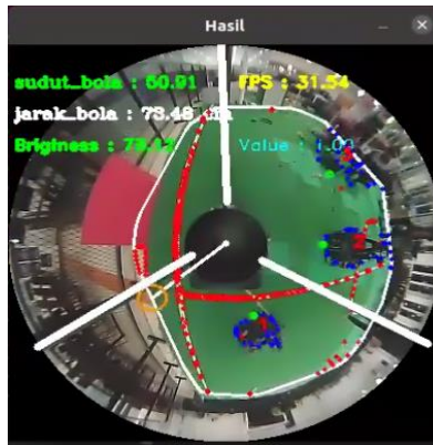
Fig. 14 Detection results using an omnidirectional camera
