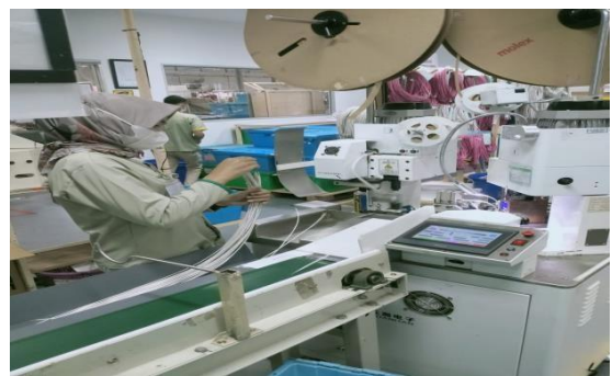
Figure 3.2 Cable cutting process on an auto cutting machine
