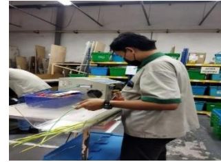
Figure 3.3 The process of cutting cables on a semi-auto cutting machine
