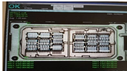
Figure 12. Standard Measure of Distane the Gluing on the module
