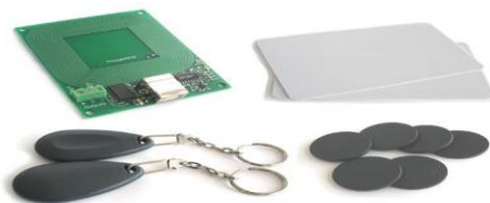
Gambar 4.1.1 Macam-macam Tag RFID
