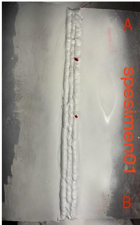
Gambar 8. Hasil Penetrant Test Specimen 1
