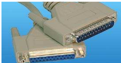
Gambar 3.7 Kabel Port paralel
