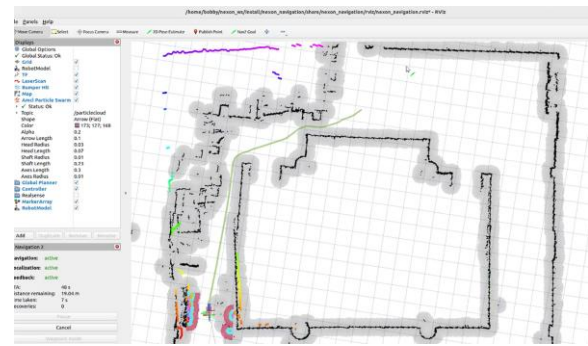
Figure 4. RViz visualization of the autonomous navigation process showing the global path, local trajectory, and robot pose during a delivery task.
