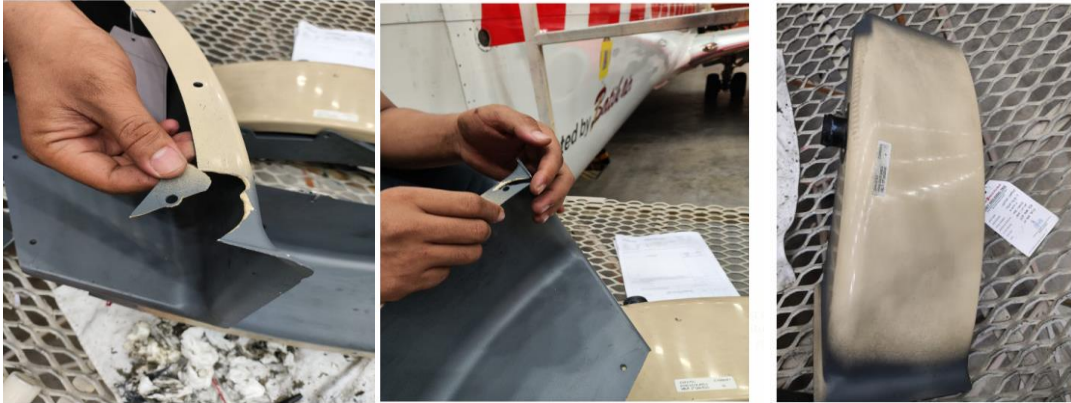
Gambar 6 : crack upper shroud
