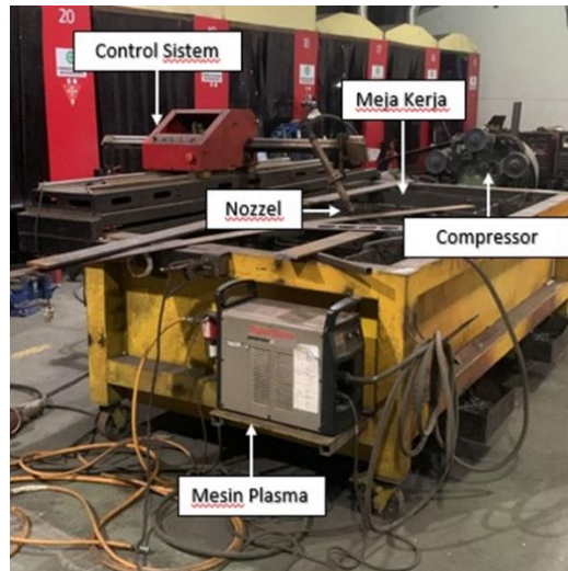
Gambar 10 : Mesin plasma cutting
