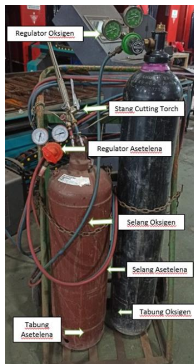
Gambar 7 : Peralatan cutting torch
