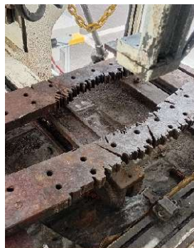
Gambar 1.1 Kerusakan Worktable/Bar Support akibat Overcutpath
