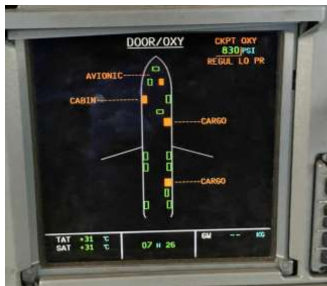
Gambar 2. Indikasi Pengoperasian Cargo Door Di ECAM
