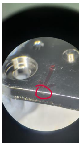
Gambar (h). Defect “Yellow stain at edge”
