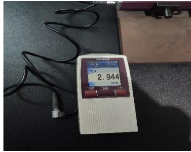
Gambar 3. Hasil kalibrasi alat surface roughness
