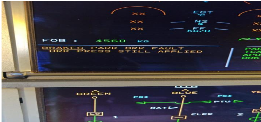
Gambar 5: Indikasi fault parking brake di ECAM
