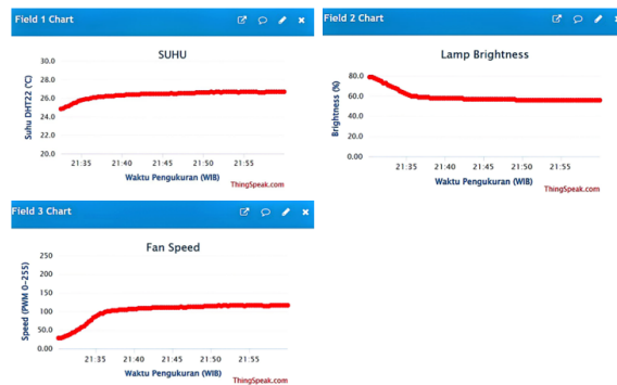
Figure 15. Graph on ThingSpeak Showing Real-Time Temperature Monitoring and Control on 4 chickens.
