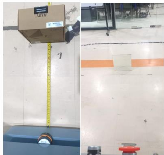
Figure 5 Position of Test Objects Relative to Sensors at Specific Distances, such as 1 m and 2 m
