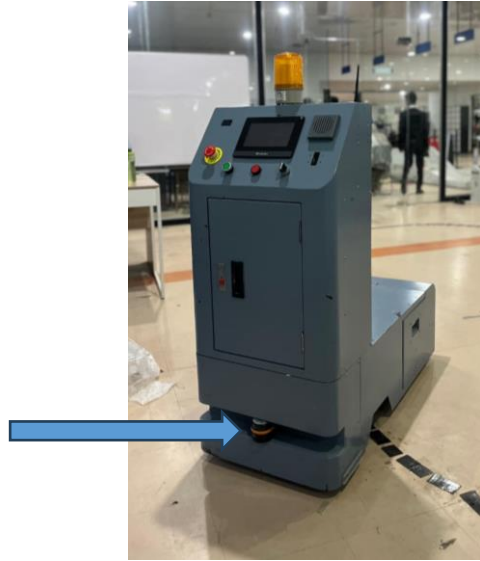
Figure 2 Installation of LiDAR sensors on AGVs
