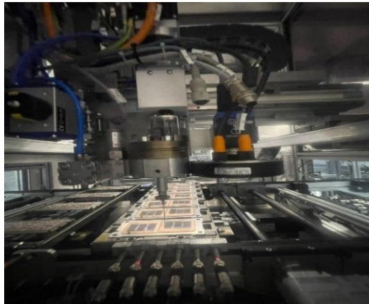
(b) Glue installation process
