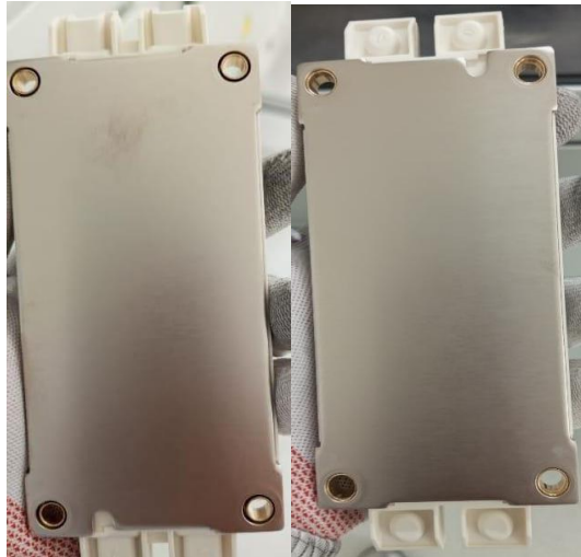
Figure 19. Shows the module before and after the rivet clamping process.
