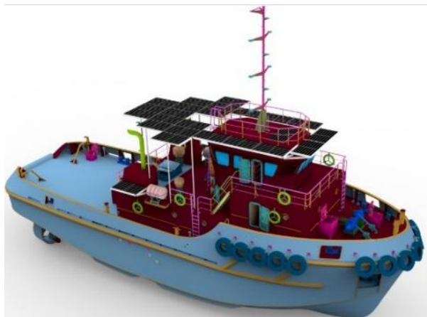
Gambar 4. Isometric peletakan photovoltaic
