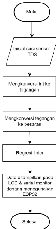
Gambar 11 Flowchart program sensor TDS
