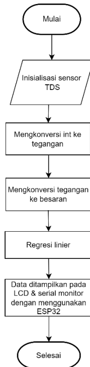
Gambar 11 Flowchart program sensor TDS
