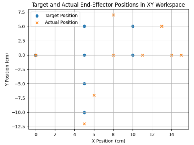
Figure 2. Distribution of target and actual end-effector positions in the XY workspace
