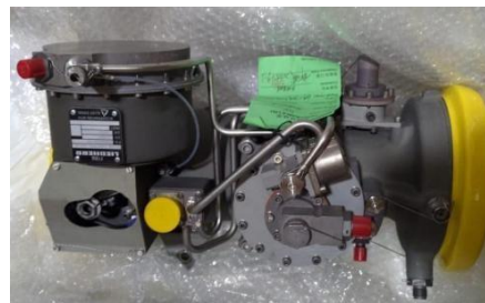
Gambar 9 Part Repaired (Valve- Flow Control)
