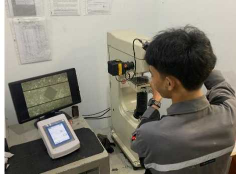
2. Proses Hardness Vickers testing (non PWHT)
