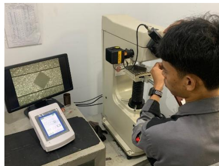
4. Proses Hardness Vickers testing (PWHT 3 jam)
