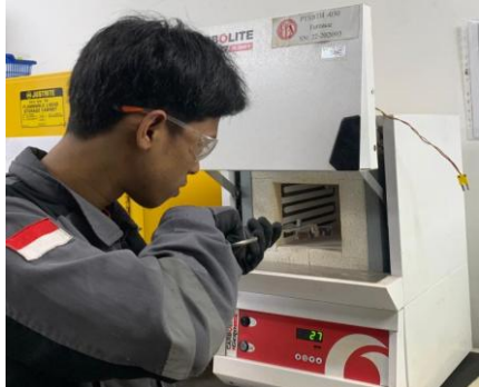
1. Proses PWHT material uji
