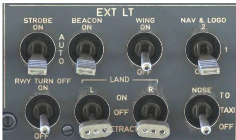
Gambar 2: exterior light switch
