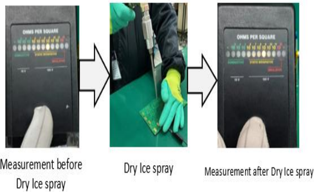
Figure 3.5. Surface Resistivity Test Results Before and After Dry Ice Cleaning
