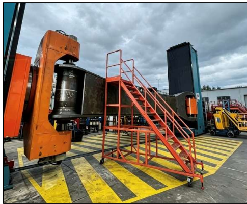
Gambar 3. Contoh Rotator Boom beserta Platform Ladder
