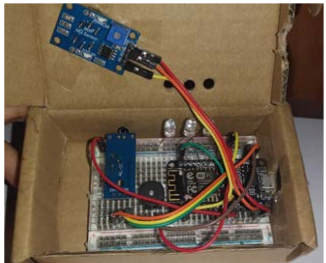
Fig. 7. The gas leak detection device
