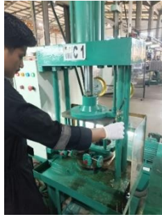
Gambar 4: Testing katup butterfly 700Z
