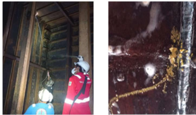
Gambar 5: Proses (a) Air Test dan (b) Porosity
