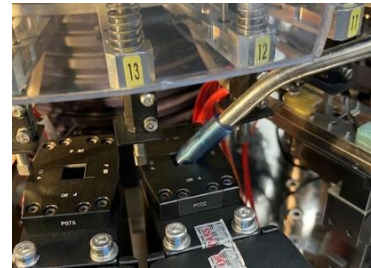
Figure 8. Air Gun Nozzle Inserted into the Top Mirror Vision Area During Cleaning
