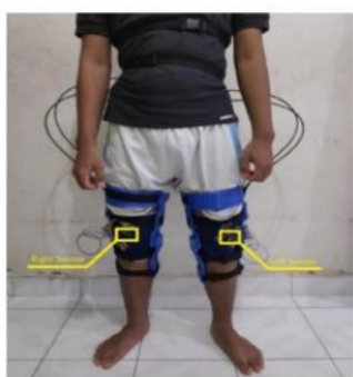
Fig. 1. The mechanical design of the knee joint lower limb exoskeleton of the (a)front view, (b)top view, (c)3D overview of knee joint design(d)prototype of the knee joint by front view, (e)prototype by side view.
