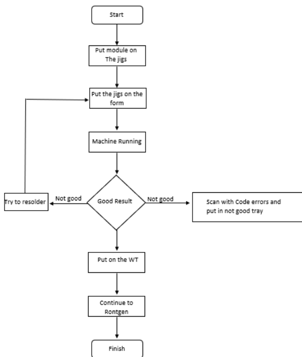
Figure 1. Flowchart of process soldering
