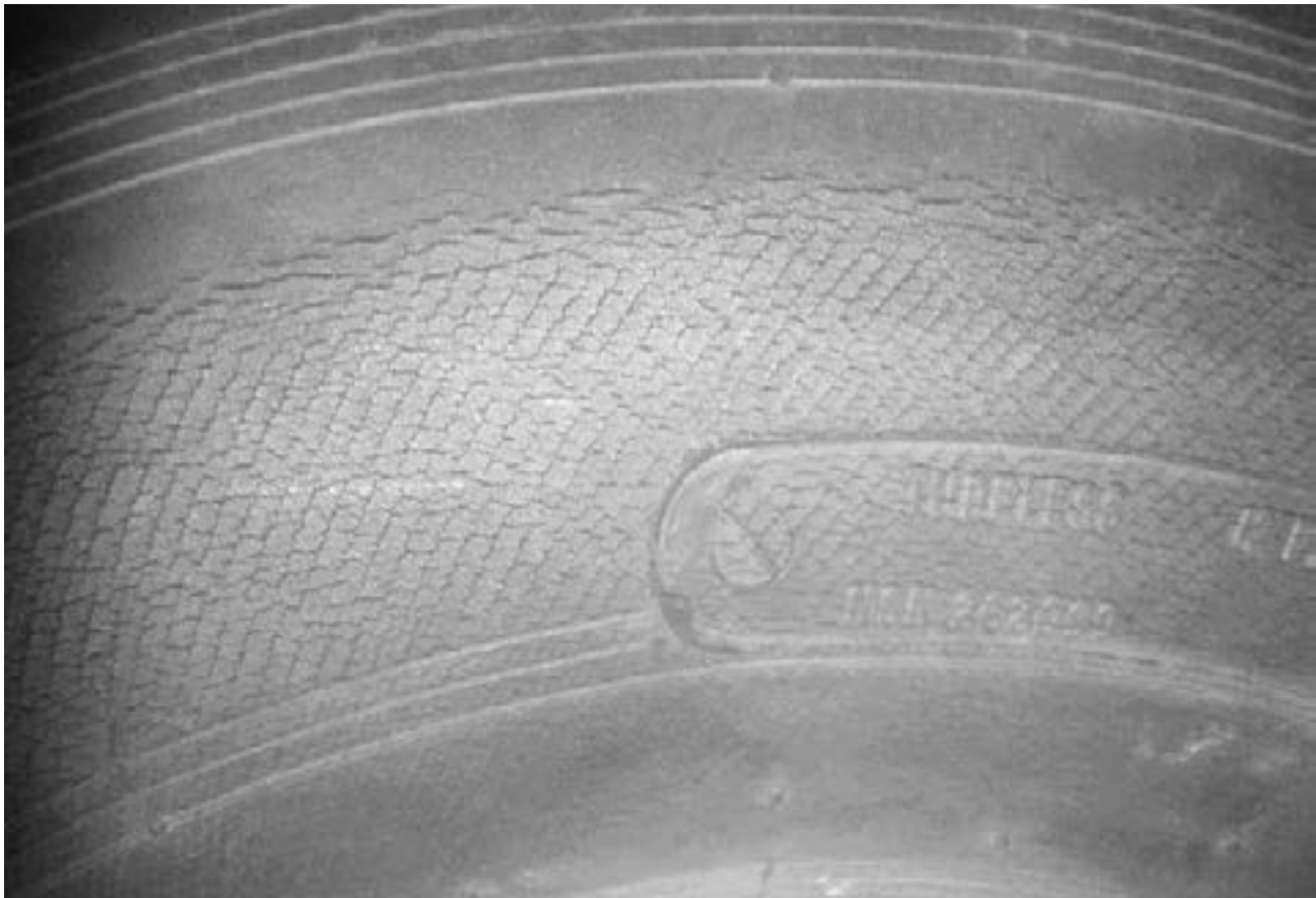
SIDEWALL CRACKING FIGURE 21
