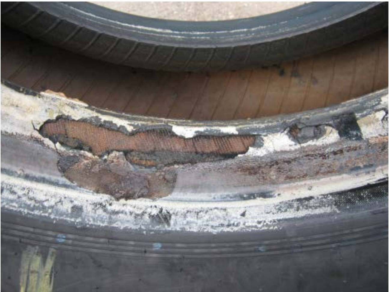
HIGH BRAKE HEAT FIGURE 23
