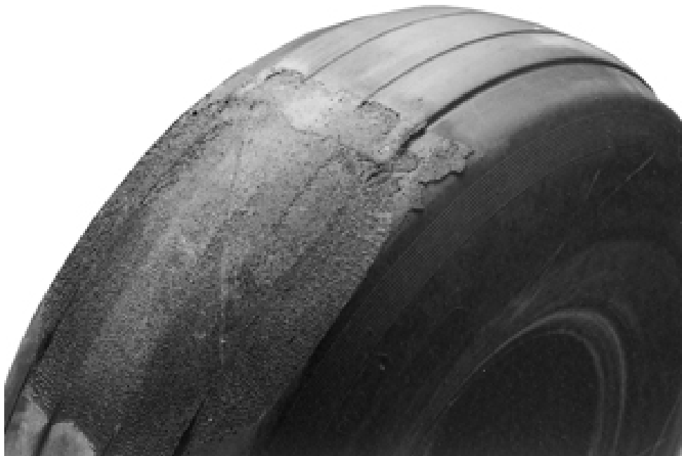
WET BRAKING FLATS FIGURE 16
