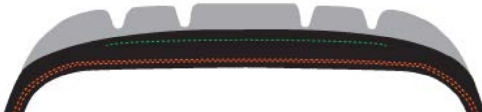
WEAR BELOW TREAD GROOVES FIGURE 31
