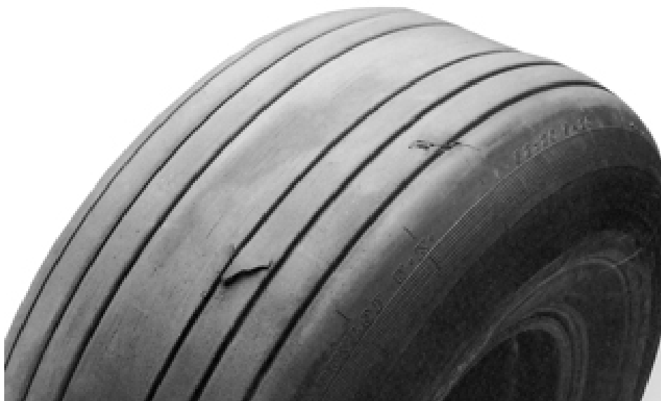
CUT DAMAGE FIGURE 14
