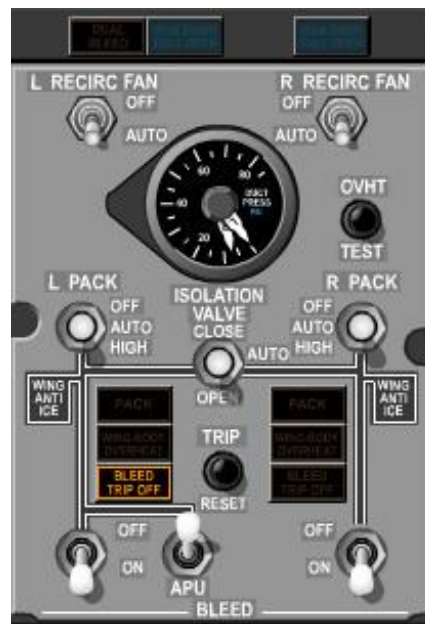
Gambar 2. Air Conditioning/Bleed Air Control Panel
