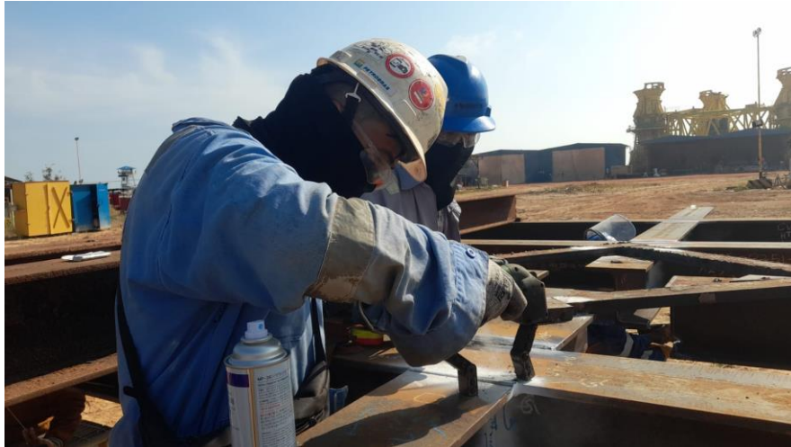
Gambar 6. Proses Magnetic particle testing (MT)
