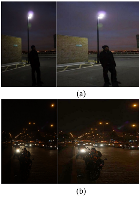
Figure 4. Comparative visualization of Zero-DCE enhancement: (a) Original low-light images from ExDark; (b) Corresponding Zero-DCE enhanced images showing improved brightness, contrast, and object visibility without overexposure artifacts.
