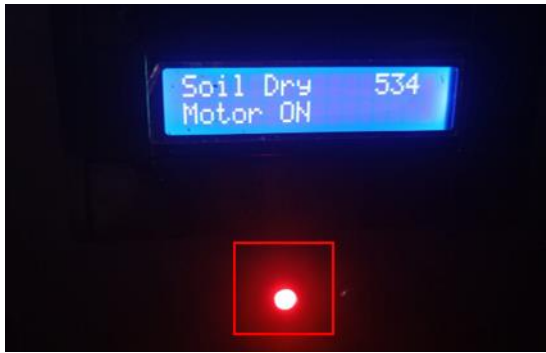
Gambar 17. Tampilan LED Saat Tanah Kering
