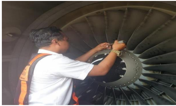
Gambar 6a : Balance screw solution inspection check
