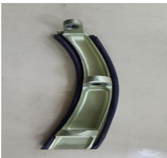
Gambar 7c : Platform seal serviceable condition
