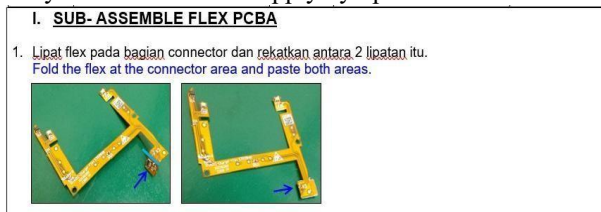
Figure 3. Work Instruction Flex PCBA Before Update
