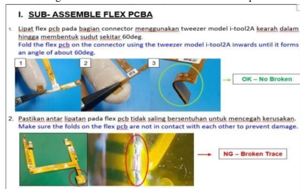
Figure 4. Work Instruction Flex PCBA After Update
