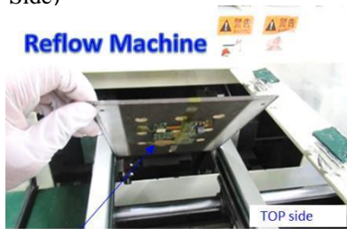
Figure 21. Put the top side PCB to SMT pallet
