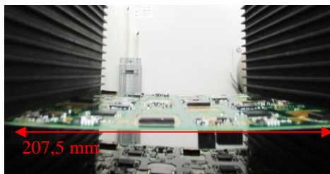
Figure 8. NG PCB Warping not using stiffener
