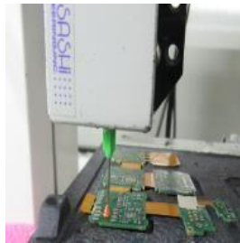
Figure 13. Machine nozzle during epoxy bonding
