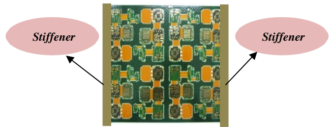
Figure 9. Illustration of stiffener addition
