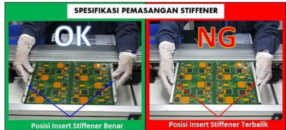
Figure 32. Stiffener installation specifications
