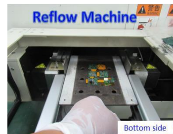
Figure 19. Put the bottom side PCB to SMT pallet
