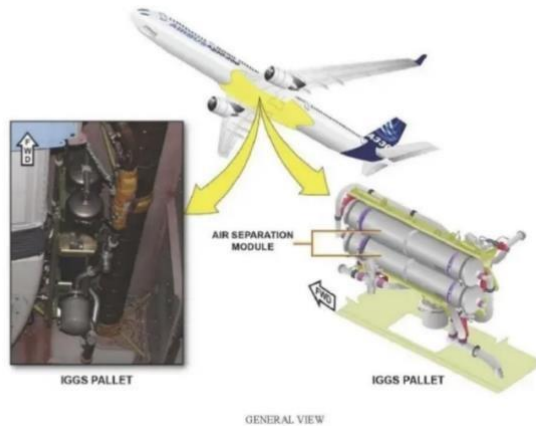
Gambar 1. Inerting Gas Generation System (Sumber : aircraft training manual Airbus 330-900, ATA 47)
