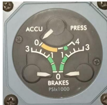
Gambar 4 : Indikasi Accumulator pressure pesawat Airbus A330-300 [5]
