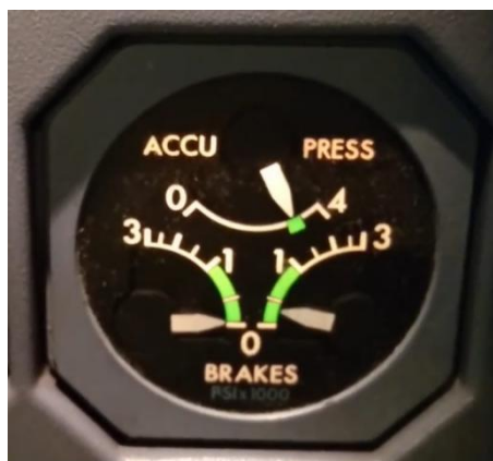
Gambar 9 : Triple pressure indicator [10]
