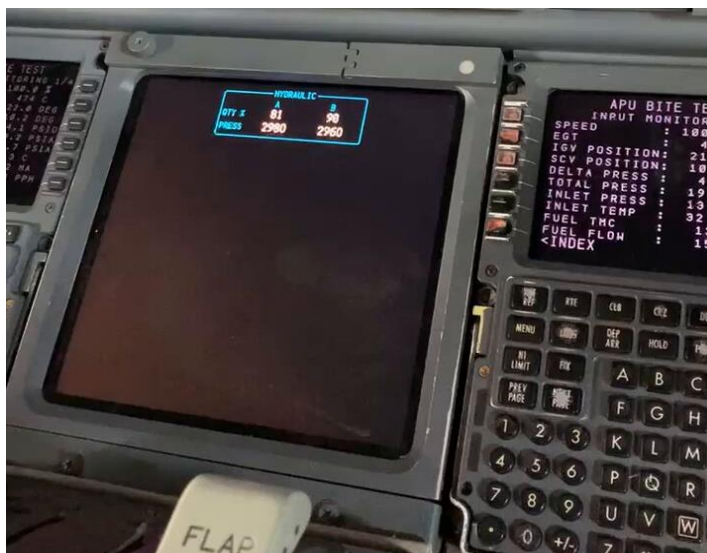
Gambar 1 : lokasi Hydraulic Fluid Indication System .
