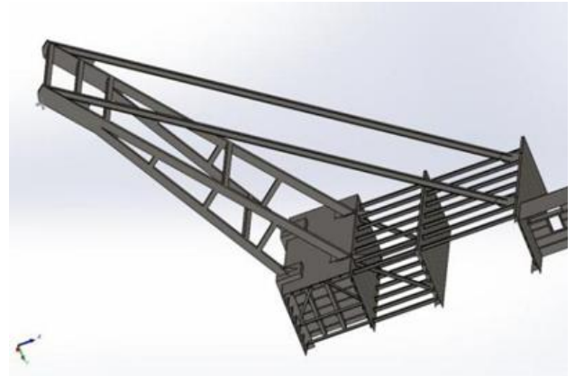
Gambar 6(b) A-frame install to barge
