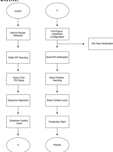
Figure 7. Machine Setup Procedure Showing The Absence of a Dedicated Glue Verification Step Before Production Release
