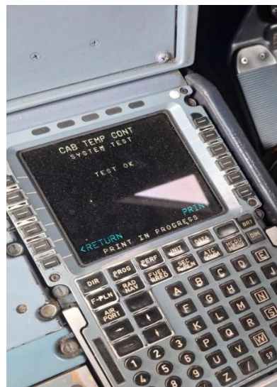
Gambar 6. Verifikasi hasil pasca packing seal replacement
