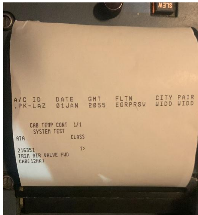
Gambar 2: report MCDU, fault trim air valve
