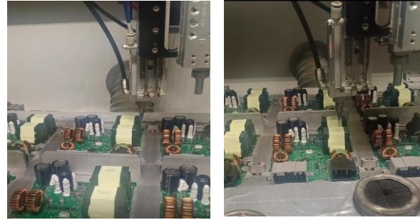
Figure 4.1 shows the PCB coating process using a selective coating machine on a production line. The coating process is carried out using a controlled spray method using a nozzle that moves along a predetermined path. In this process, the PCB is positioned on a jig to ensure stability during the coating process.
